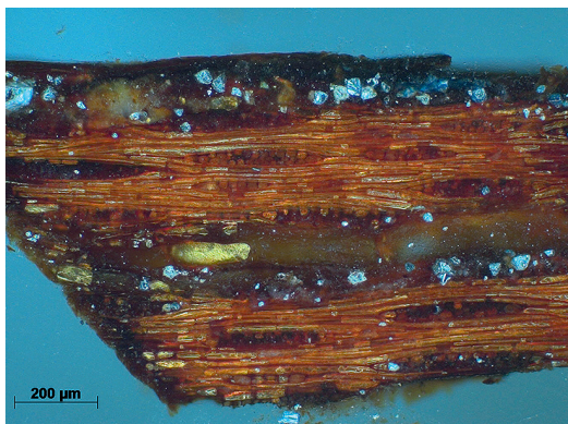
Figure 3 Cross-section of finish sample from the chest on chest. Left: visible light; right: ultraviolet light. The lack of fluorescence in the wood pores suggests a wax original coating. Photo by Stephanie Auffret.
