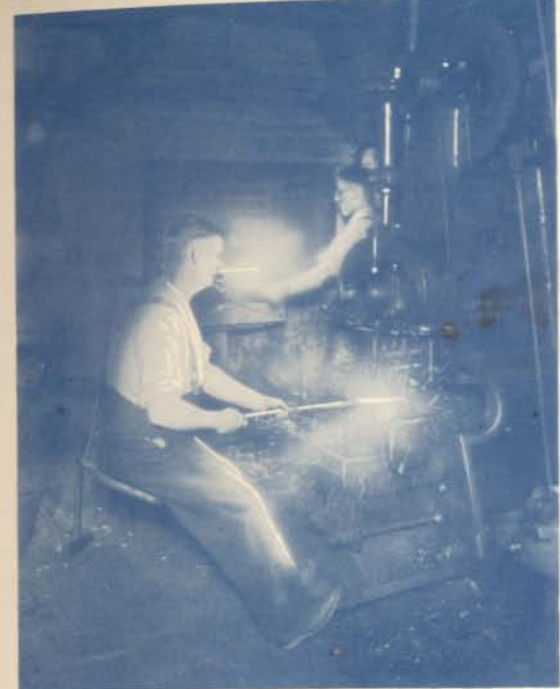
Forging MARPLES Famous Crucible Cast Steel Plane Irons.
