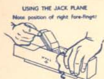
EDGE PLANING Note method of gripping plane, to keep the edge square
