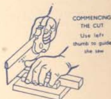
CROSS CUTTING Support the outer end with left hand
