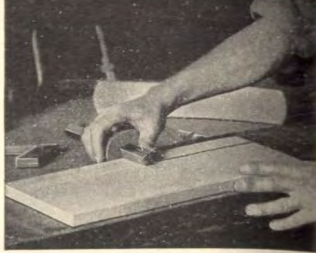
Scribing with a marking gauge
