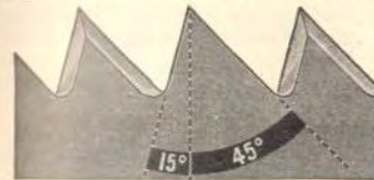
Side view of cross-cut teeth (enlarged)
