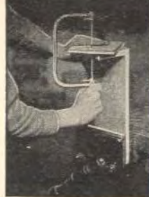
Using coping saw with saddle
