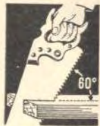
Proper angle for ripping
