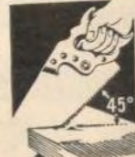
Proper angle for cross-cutting
