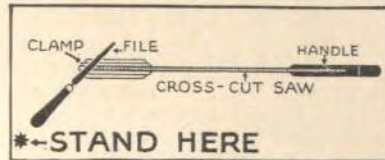
First position for filing hand saws for cross-cutting
