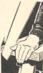
Starting the cut with a draw stroke
