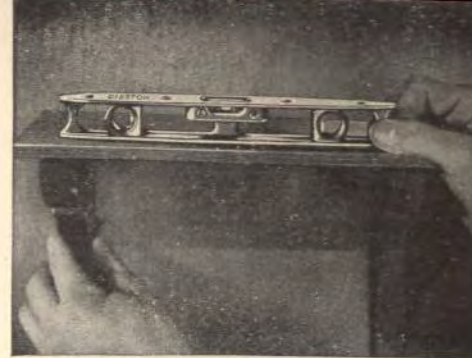
Leveling shelf with Disston A-10 Level
