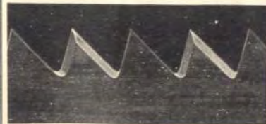
Shape of cross-cut saw teeth
