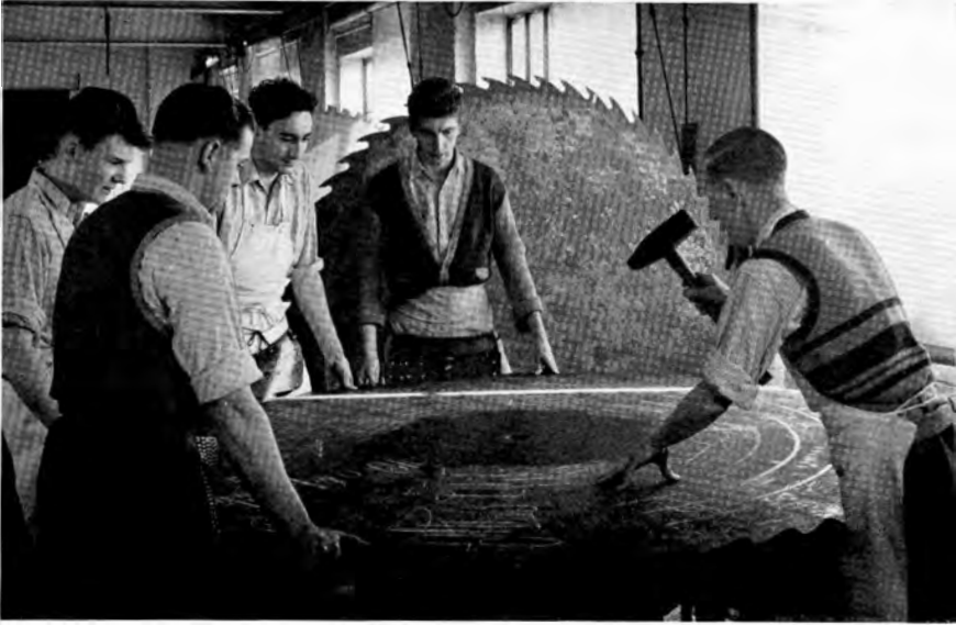
74. Smithing: putting the tension into a saw blade. An 84-inch diameter solid tooth saw is shown
