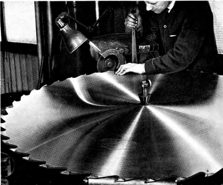
85. Final lapping by diamond impregnated wheel of a 50-inch diameter tungsten carbide-tipped saw
