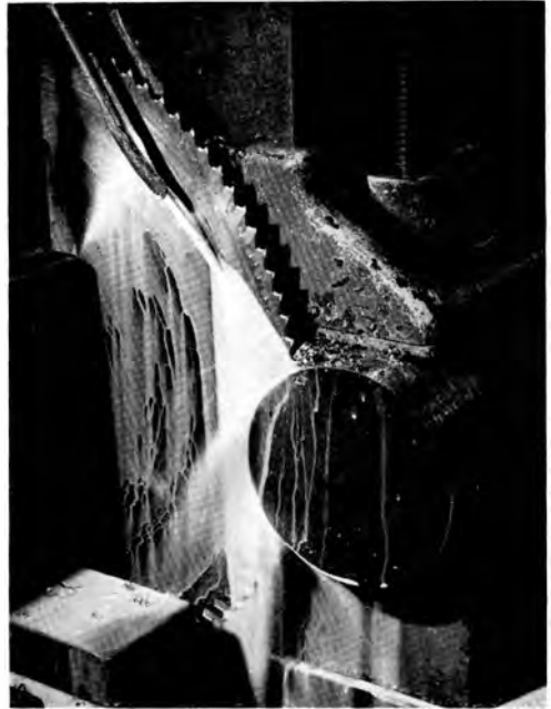
81. Cutting cold metal by segmental circular saw
