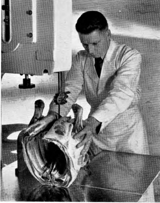
91. Abattoirs use bandsaws for cutting carcasses. Smaller bandsaws, such as this Wadkin-Bursgreen machine with 16-inch wheels, are found useful by retail traders for cutting meat into small joints
