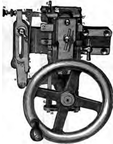
Fig. 347. Prybil's Band Saw Setter.
