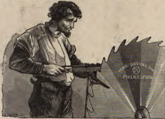
Fig. 187. Saw Filing Machine.
