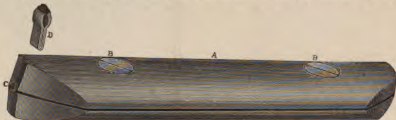
Fig. 216. Emerson's Diamond Tool for Truing Wheels.
