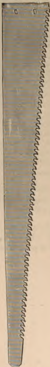
Fig. 302. Pit Saw Blade.
