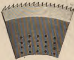
Fig. 88. Cutting Segment of Circular Saw.
