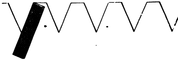
Fig. 249. Flat File on Peg Teeth.
