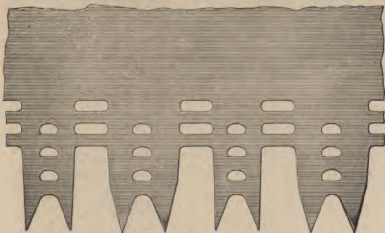
Fig. 54. Perforated Cross Cut.
