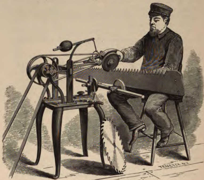
Fig. 277. Frey's Gummer and Sharpener for Straight Saws.
