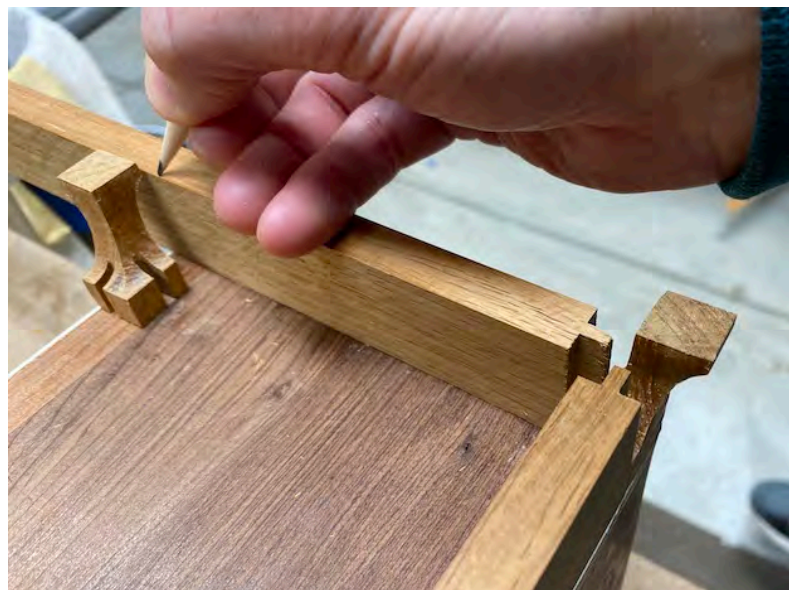
Put the tenon in one leg/foot and mark approximate other end of tenon so skirt board will space the feet the correct distance apart. (Note the skirt hasn't been shaped yet so it looks over-wide)
