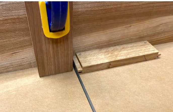
The picture below shows placement to shave a bit off the tenon end.
