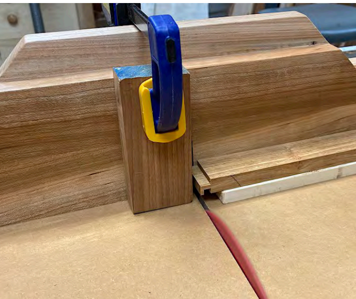
Use a stop block and spacer board to dial in the tenon thickness. The stop block ensures perfectly aligned shoulders.
