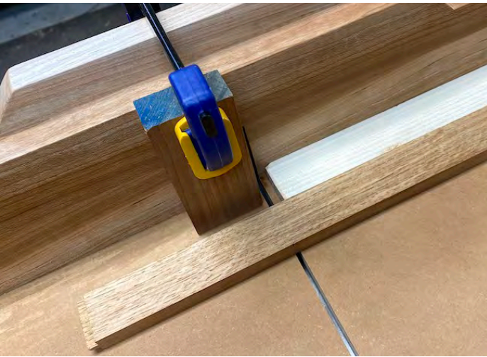
Now you can remove the same spacer board to let you trim the skirt to that marked length, without having to remove the stop block.
